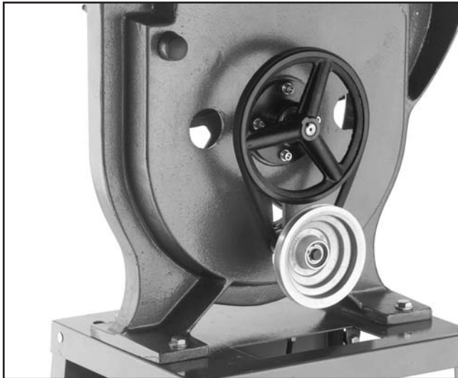
Figure 14. Stepped pulley installed with wheel pulley V-belt in place.
